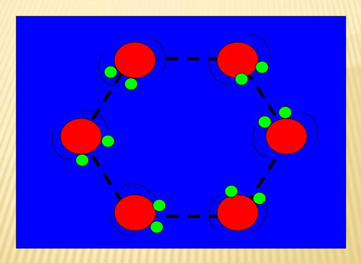
When water molecules are cooled they move slowly and attach to each other forming these 6 sided (octagonal) ice crystals. Freeze-Point-Depressant – Is a material that has been used to prevent precipitation and condensation from freezing as quickly as it otherwise would have. (It is the ability to lower the freezing point of water.)
