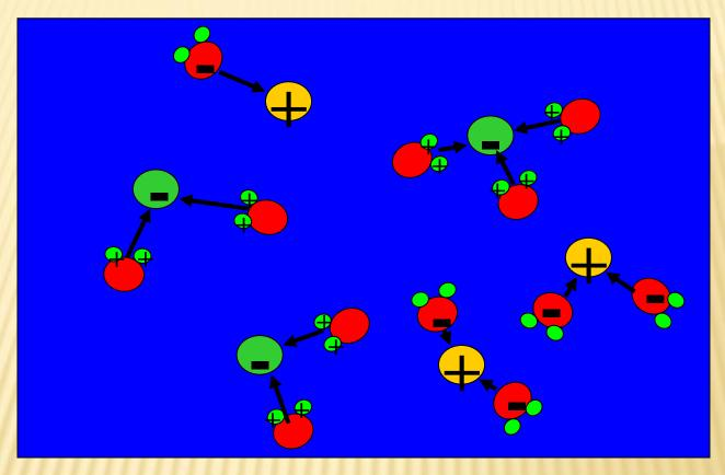
When salt is applied to snow/ice the positively charged sodium atom attracts the negatively charged oxygen atom and likewise the negatively charges chloride atom attracts the positively charged hydrogen atoms, causing the 6 sided ice crystal to break apart.
